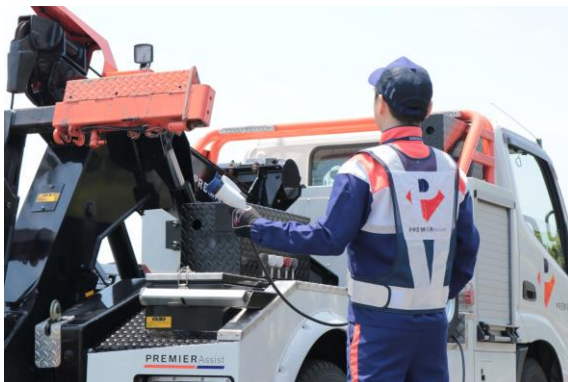
Tow trucks capable of supplying power to EVs
